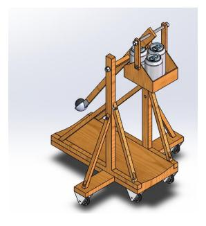
Using SolidWorks I produced a quick design of some of the requirements of the project. The mass includes the shape and size of the 3 soda cans that would be used in the real life product. The only thing that could not be produced was the sling that would be attached to the end of the swing arm to allow for the projectile to track its' course of motion.
